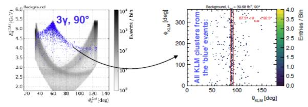
Cosmics + Phase 2 e<sup>+</sup>e<sup>-</sup> $\rightarrow$ µ<sup>+</sup>µ<sup>-</sup> $\gamma$  will be used to get detailed maps of gaps and materials (cables, pipes, ...) inside the gaps
