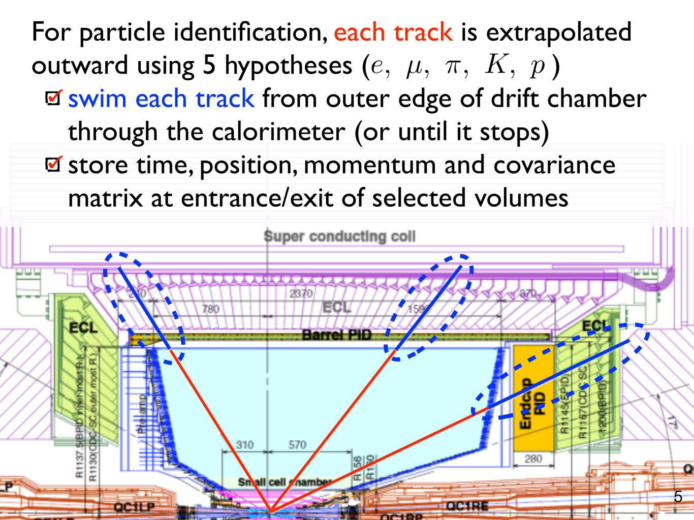
For muon identification, each track is extrapolated outward using µ hypothesis (but could use the other 4)
