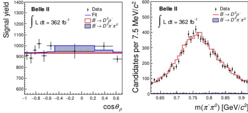
**Figure 2:** Left: background-subtracted  $\cos \theta_\rho$  distribution with fit projection overlaid. Right: background-subtracted distribution of the  $\pi^- \pi^0$  invariant mass, with overlaid simulated data reflecting the  $B^+ \rightarrow D^0 \rho^+$  and  $B^+ \rightarrow D^0 \pi^+ \pi^0$  proportions from the  $\cos \theta_\rho$  fit
