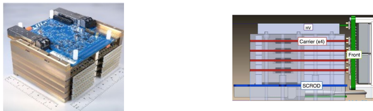
Fig. 4. TOP boardstack consisting of one SCROD board, four AISC boards and one HV supply module.
