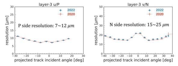
**Figure 3:** Distribution of position resolution for p-side (left) and n-side (right) as a function of the incident angle. Comparison between data taken in 2020 (dots) and 2022 (dotted line) is presented.
