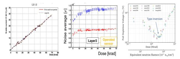
**Figure 4:** Left plot: Leakage current as a function of the accumulated dose; Center plot: the average noise level as a function of accumulated dose for p-side (blue dots) and n-side (red dots); Right plot: full depletion voltage as a function of the accumulated dose with the type inversion observed at 2 Mrad.
