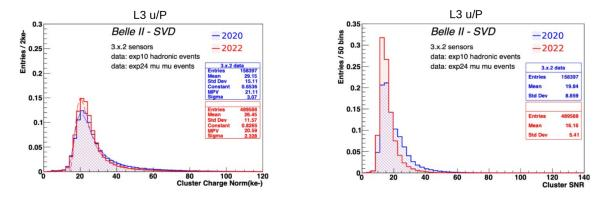
**Figure 2:** Distribution of Cluster Charge (left) and Signal-to-Noise Ratio (right) for Layer 3 (p-side). Comparison between data taken in 2020 (blue) and 2022 (red) is presented.
