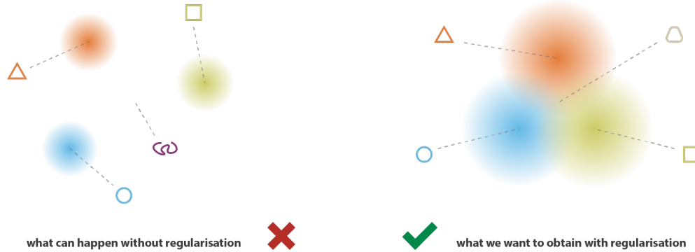
Figure 4.2.: The figure depicts the continuity and completeness of latent space. The image on the left shows the distributions of different classes that are encoded far apart in the latent space, giving meaningless output during interpolation. This image lacks continuity and completeness. The image on the right shows an encoded latent space of different classes with overlapped distributions which is complete and continuous [43].
