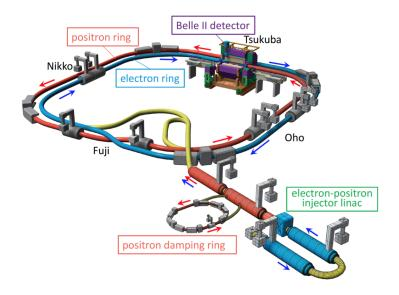
Figure 1.3: Schematic view of the Belle II experiment at the SuperKEKB accelerator. [AFK18]
