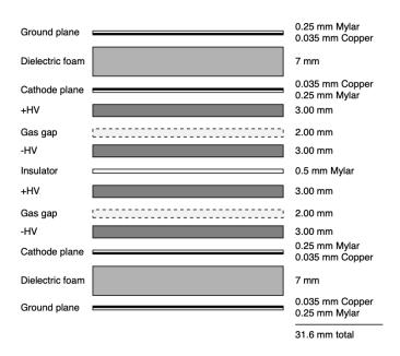
Figure 1.5: Profile of a RPC superlayer used in the barrel of the Belle II KLM. [Abe+10]
