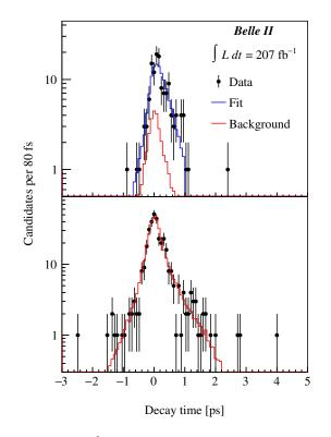
**Figure 3:** Decay-time distributions of  $\Omega_c^0 \to \Omega^- \pi^+$  candidates in their (top) signal and (bottom) sideband regions with fit projections overlaid.
