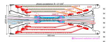
Figure 1: Schematic cross-sectional view of the VXD. The SVD is red, the PXD is light blue, and the IP beam pipe diamonds are pink circles. In the upper <sup>62</sup> half of the VXD the locations of the three types of SVD DSSDs are indicated <sup>63</sup> by boxes in three colors: purple for small sensors, green for large sensors, and <sup>64</sup> orange for trapezoidal sensors as described in Tab. 1.
