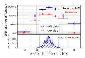
Figure 5: The relative hit efficiencies (the ratios of the hit efficiency in the three-207 samples data to the one in the six-samples data) as a function of the trigger timing shift for v/n-side (blue square) and u/p-side (red diamond). The positive (negative) trigger timing shift corresponds to early (late) trigger timing.
