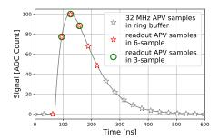
Figure 2: Example of sampling in "multi-peak" mode of the APV25. The gray line shows the signal waveform after the CR-RC shaper circuit. The stars show the sampled signal height recorded in the analog ring buffer according to the 32 MHz sampling clock. The red stars indicate the six successive samples read out at the trigger reception in the six-samples mode. The red stars with a green circle indicate the samples read out in the three-samples acquisition.
