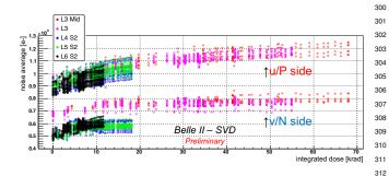
Figure 7: Effect of the integrated dose on the noise average in electron. The  $_{314}^{313}$  upper (lower) series shows the u/p-side (v/n-side) results, respectively.
