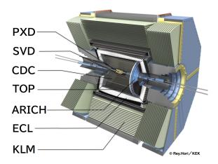
Figure 1: The Belle II detector.
