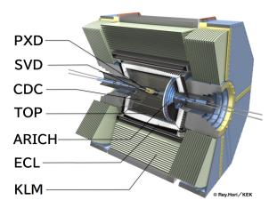
Figure 1: The Belle II detector.
