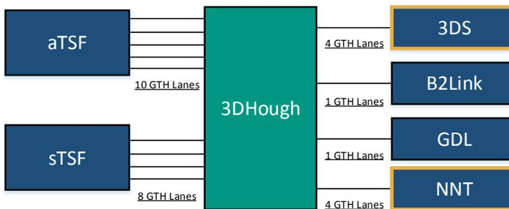
Figure 6.1.: Block diagram of the S3D describing all required input and output interfaces with the number of respective required GTH lanes. Interfaces depending on the integration method are highlighted orange.
