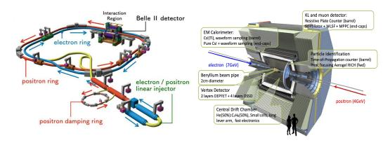
Figure 1: SuperKEKB accelerator (left) and Belle II detector (right).
