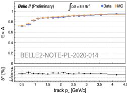
Figure 2: K-identification efficiencies and  $\pi$ -misidentification rates for different PID criteria using the decay  $D^{*+} \to D^0[K^-\pi^+]\pi^+$  (left), measured tracking efficiency times detector acceptance ( $\epsilon \times A$ ) and calibrated data-MC discrepancy ( $\delta^*$ ) for the combined channels as a function of the 1-prong track  $p_T$  (right).
