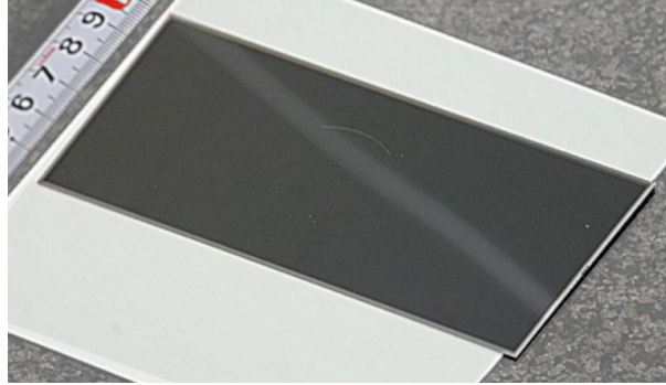
Fig. 1.5: A photo of a DSSD sensor. This type of sensors are used in L4–6 parallel regions (drawn in green color in Fig. 1.3).
