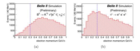
Fig. 1. Momentum distributions of low-momentum electrons coming from (a)  $B \rightarrow K^{(*)}\tau\tau$  and (b)  $\tau \rightarrow eee$  decays. The dashed vertical lines indicate the transverse momentum threshold required to reach the ECL.
