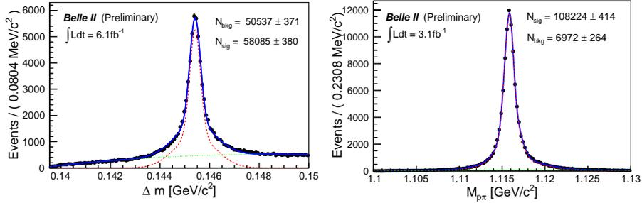
**Fig. 1.** Fitted distributions of  $\Delta m$  from the  $D^*$  sample (left) and of  $M_{p\pi}$  from the  $\Lambda$  sample (right). The size of the dataset used for  $D^*$  calibration is larger to have enough low momentum kaon tracks.
