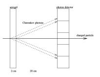
Figure 3.13: Proximity focusing ARICH - principle
