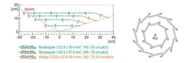
**Figure 3.9:** Left: Schematic view of the SVD longitudinal section, showing the sensors geometry for each layer and the number of APV25 chips on each side of the sensors. Right: the windmill structure of the inner sensors, with the Origami concept applied on the upper edge of silicon modules, is shown.
