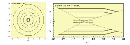
**Figure 3.7:** A shematic view of the Belle II vertex detector, two pixelated layers and four layers with silicon strip sensors
