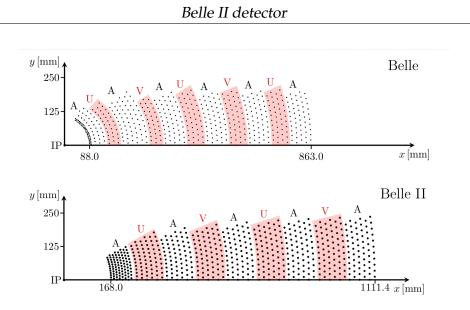
**Figure 3.8:** Layer configuration of the CDC at Belle (top) and at Belle II (bottom). The letter A stays for axial superlayers; the letter U for stereo superlayers with positive stereo angle; and the letter V for stereo superlayers with negative stereo angle.
