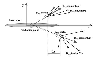
Figure 4.1: Principle of TDCPV measurment.
