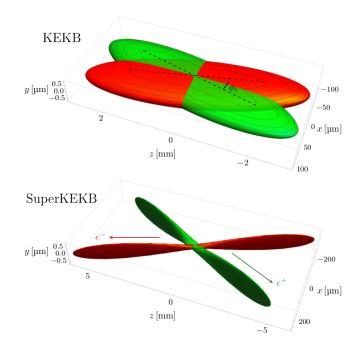
**Figure 3.3:** Schematic view of the beam crossing at KEKB (top) and at SuperKEKB (bottom). The crossing angle is shown in the top. The beam directions are shown in the bottom scheme. The size of the interaction region in z-direction at KEKB was around 10 mm, while at SuperKEKB it is around 0.5 mm
