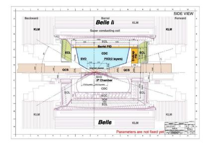
**Figure 3.6:** Illustration showing in the top, the upgraded Belle II detector as designed in the Belle II Technical design report [34], while in the bottom, the longitudinal view of the old Belle detector is shown.
