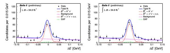
**Figure 2:** Distribution of  $\Delta E$  for  $B^0 \to K^+\pi^-$  (left) and  $\overline{B}^0 \to K^-\pi^+$  (right) decays with fit projections overlaid.
