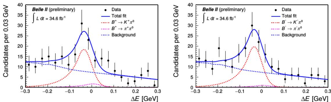
**Figure 3:** Distribution of  $\Delta E$  for  $B^+ \rightarrow K^+ \pi^0$  (left) and  $B^- \rightarrow K^- \pi^0$  (right) decays with fit projections overlaid.
