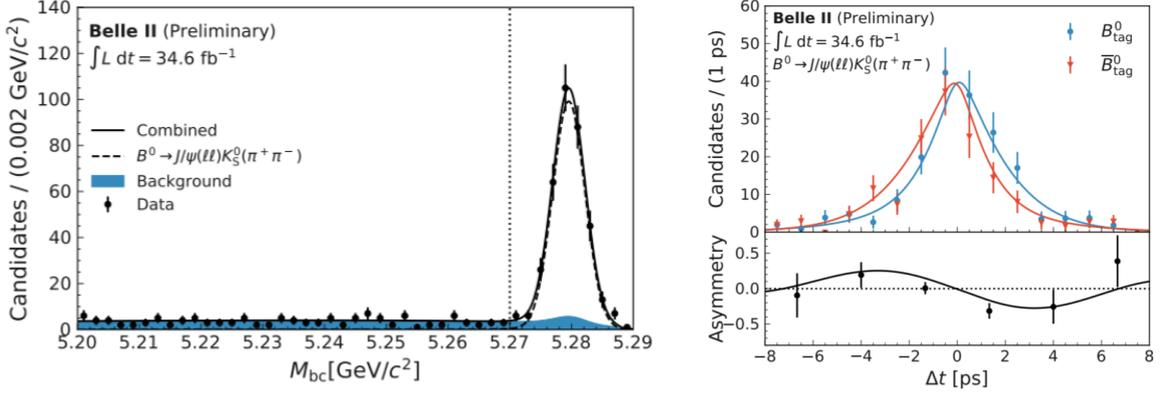
**Figure 6:**  $M_{bc}$  distribution with fit projection (left) and background subtracted  $\Delta t$  distribution and asymmetry as a function of  $\Delta t$  for the channel  $B^0 \rightarrow J/\psi K^0$ .
