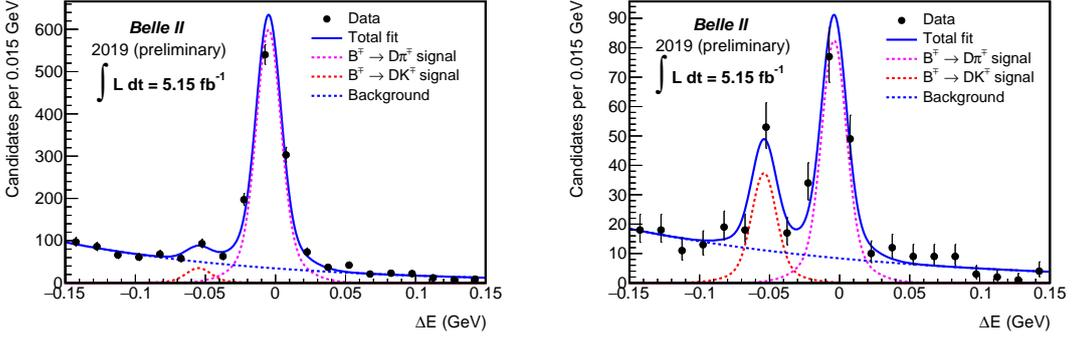
**Figure 3:** Distributions of  $\Delta E$  for  $B^- \rightarrow D^0 h^-$  without PID criteria (left) and with PID requirement (right) ( $h = \pi$  or  $K$ ) candidates reconstructed in  $5.15 \text{ fb}^{-1}$  of collision data with the projection of an unbinned maximum likelihood fit overlaid.
