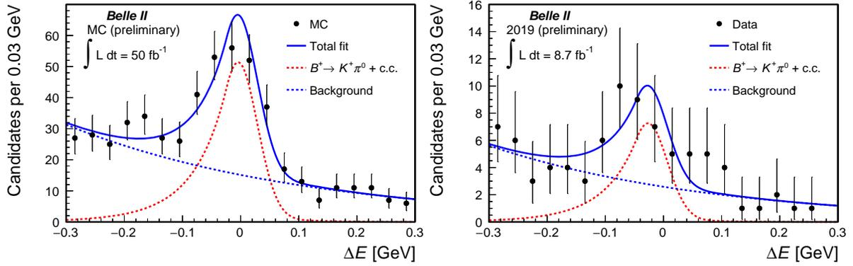
FIG. 4. Distributions of  $\Delta E$  for  $B^+ \rightarrow K^+ \pi^0$  candidates reconstructed in (left) simulated data and (right) 2019 Belle II data, selected through the baseline criteria plus an optimized continuum-suppression, kaon- and  $\pi^0$ -enriching selection, further restricted to  $M_{bc} > 5.27 \text{ GeV}/c^2$ . The projection of an unbinned maximum likelihood fit is overlaid.
