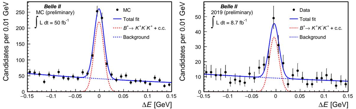
FIG. 5. Distributions of  $\Delta E$  for  $B^+ \rightarrow K^+ K^- K^+$  candidates reconstructed in (left) simulated data and (right) 2019 Belle II data, selected through the baseline criteria plus an optimized continuum-suppression and kaon-enriching selection, further restricted to  $M_{bc} > 5.27 \text{ GeV}/c^2$ . The projection of an unbinned maximum likelihood fit is overlaid.
