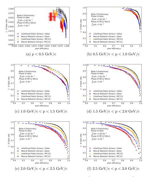
FIG. 1: pion efficiency vs Kaon fake rate with 2.62 fb<sup>-1</sup> data sample and 5 fb<sup>-1</sup> MC12 sample in each momentum region. These efficiency and fake rate are calculated by using the decay  $D^{*+} \rightarrow [D^0 \rightarrow K^- \pi^+]\pi^+_{slow}$ . Further detail is described in BELLE2-NOTE-TE-2020-005.
