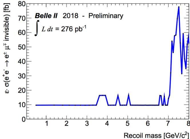
**Figure 3.** Belle II limits on the  $\varepsilon \cdot \sigma$  (where  $\varepsilon$  is the efficiency) as a function of  $Z'$  mass for the LFV model. Results cannot be expressed as limits on a coupling since the efficiencies are model-dependent and no LFV  $Z'$  model currently exists.
