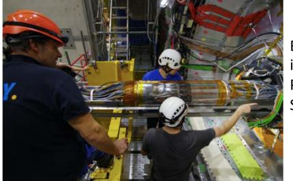
Belle II VXD ~6 layers installed on Nov 21, 2018 PXD L1 & two ladders of L2 SVD (4 layers)
