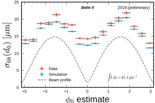
VXD resolution in impact parameter ~14 μm x2 better than Belle PXD 1st layer R=14mm
