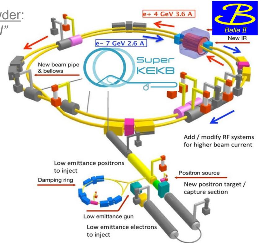
**SuperKEKB:** second generation B-Factory. It will provide the **world highest luminosity**, applying the **large crossing angle nano-beams scheme**. (P.Raimondi et al., arXiv:0709.0451)
