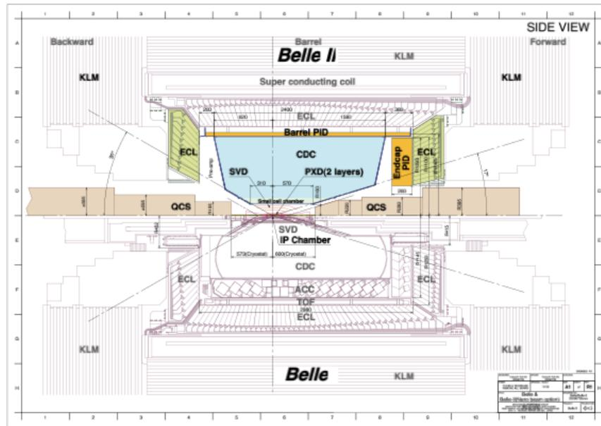
**Figure 1:** Belle vs Belle II detectors. In the top half of the drawing a side view of the Belle II detector is shown, with new or upgraded components are shown in colours. In the bottom half is the old Belle detector.
