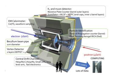
Fig. 3. – The Belle II detector.
