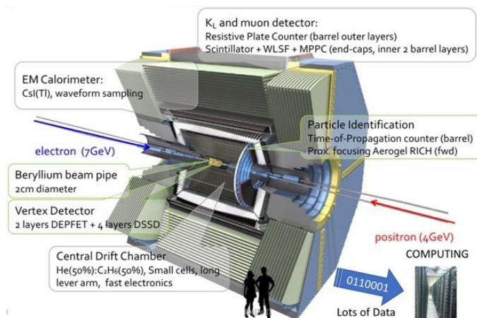
Fig. 3. – The Belle II detector.
