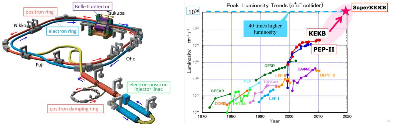
Fig. 1. – Schematic view of SuperKEKB collider (left). Luminosity profile of SuperKEKB compared with previous colliders (right).
