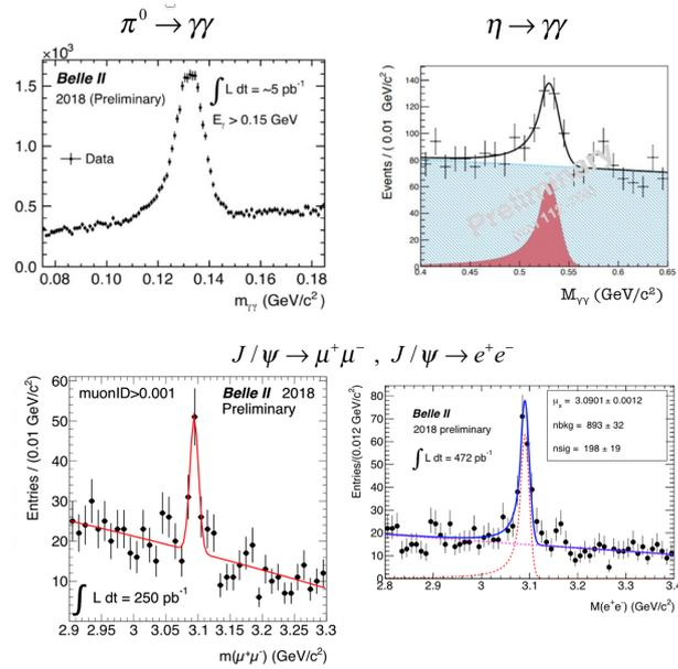
Fig. 7. – Performance of the Belle II detector during the Phase 2 commissioning run: reconstruction of  $\pi^0$  and  $\eta$  (top);  $J/\Psi$  reconstruction in muon and electron decay channels (bottom).
