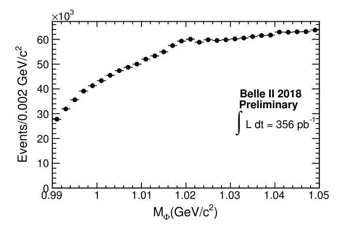
FIG. 3: This figure shows  $M[(K^+K^-)]$  distribution, which was produced using phase-II 356 pb<sup>-1</sup> prod6 hadron skim data. No PID criteria is applied on kaon tracks. Selection criteria used for reconstruction are |d0| < 2 cm, |dz| < 4 cm,  $|M(K^+K^-) - M_\phi^{\text{PDG}}| < 0.050 \text{ GeV/c}^2$  and vertex fit using two charged kaon tracks. Further details are described in the internal note - BELLE2-NOTE-PH-2018-037.
