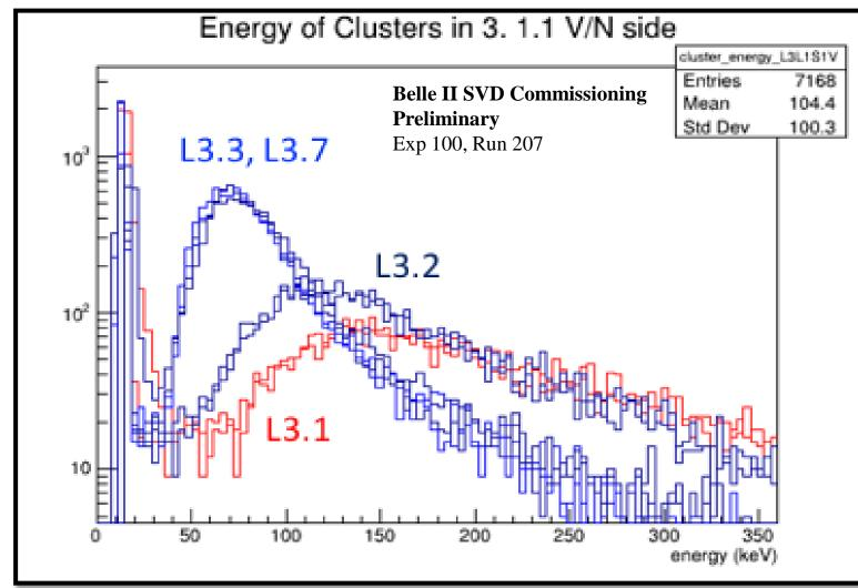
Distribution of the energy deposit in a horizontal silicon sensor (*t*=300µm) by a cosmic ray (~MIP) is peaking at 80keV. The deposit distribution for random-trigger events was peaking at ~20keV.
