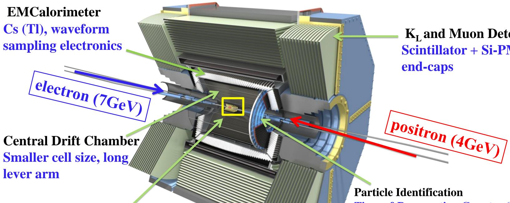
**K<sub>L</sub> and Muon Detector Scintillator + Si-PM for** end-caps
