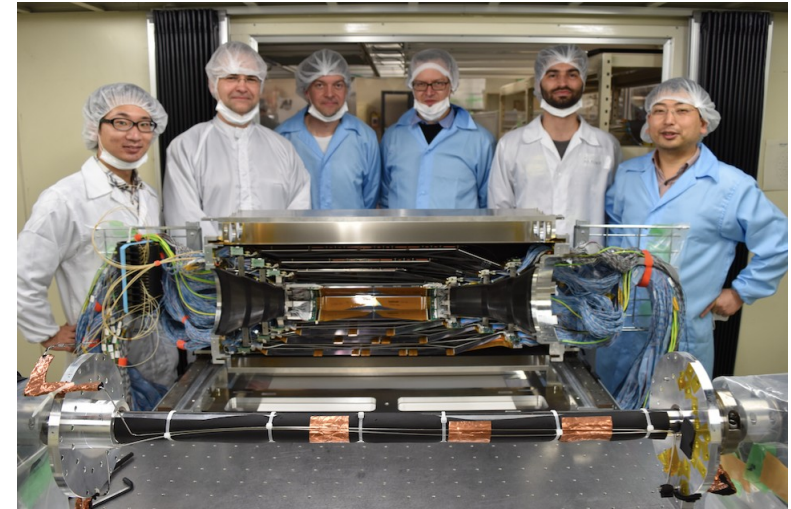
SVD half shells assembled at KEK
