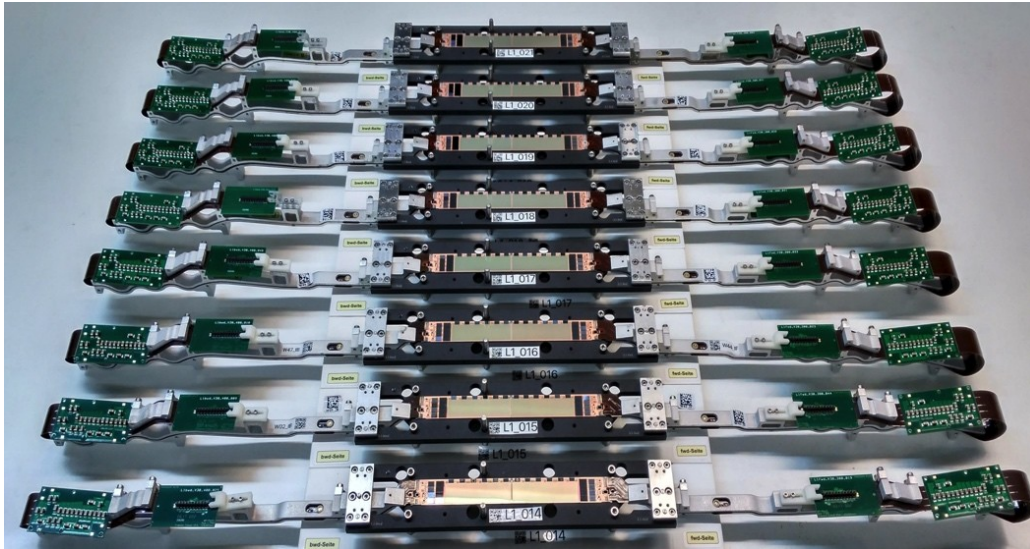
PXD ladders and assembled half shell at DESY
