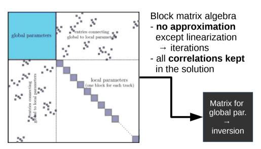
Scale of CMS tracker alignment with Millepede II (over 200k constants) ~ enough to align and calibrate "whole Belle II"  $\rightarrow$  will reduce possible weak modes (chi2 invariant distortions) in **global simultaneous fit** (cross-detector correlations kept)  $\rightarrow$  try to include as many sub-detectors as possible
