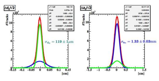
Origin of tracks in z-direction in central data reprocessing showing improving z-resolution due to better drift chamber calibration and alignment:
