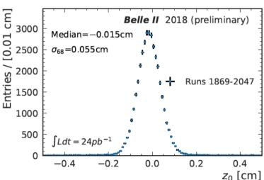
The interaction region profile in the longitudinal (z) direction, measured using the point of origin of charged particle tracks in the Belle II detector, showing the currently achieved interaction region longitudinal size of 0.55mm.
