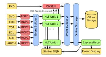
Read-out PCs (ROPC) collect and forward detector raw data to the first event builder stage.
