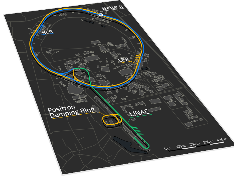
Figure 3.1: Schematic view of the SuperKEKB collider complex. Figure from Tobias Blegesen.
