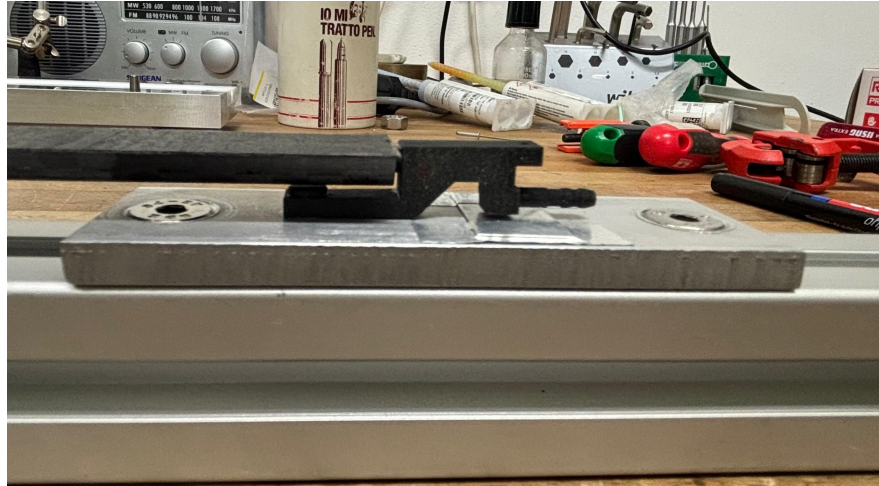
Figure 3.14: Bonding process with the kokeshi pin inserted in the housing plate fixed in the Bosh profile
