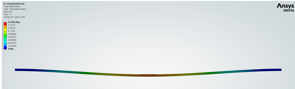
Figure 4.15: Mechanical Ansys Static Simulation with concentrated load for the ladder with 280\ \mu m of GG52 skin layer [mm].
