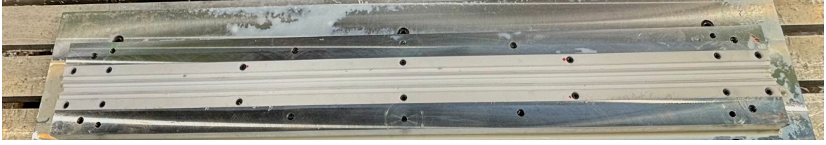
Figure 3.10: Omega beam mold after the milling process
