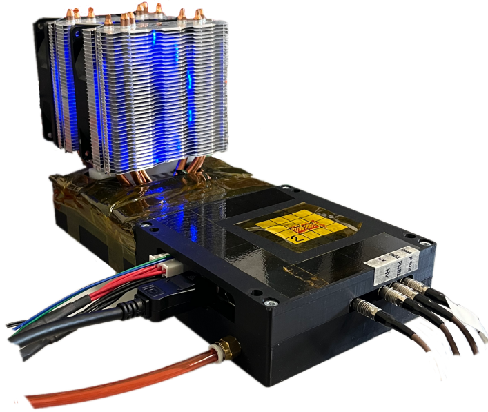
Figure 20: Peltier temperature control system housed in a custom 3D-printed casing with all necessary connections.
