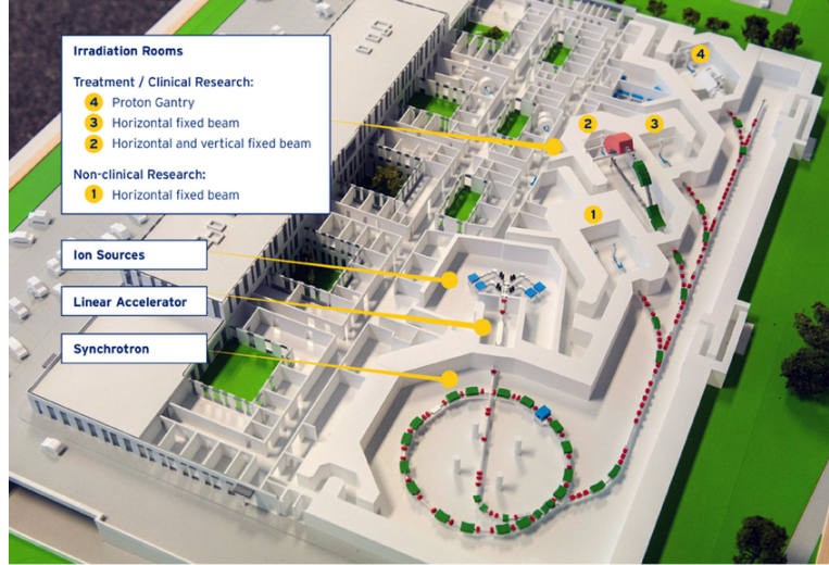
Figure 38: Schematic model of the MedAustron cancer treatment and experimental facility in Wiener Neustadt, Austria. [53]
