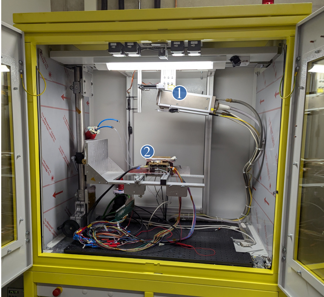
Figure 3.6: Photograph of the X-ray irradiation chamber. The X-ray tube is mounted at the top and angled downward toward the irradiation target. The Hybrid5 module is mounted on the height-adjustable rig at the center. Oscilloscope probes are connected from the back and are covered with lead shielding, while power and InfiniBand cables are routed from the sides. Cooling fluid circulates through transparent tubes from front to back. A brass shield with cutouts for the DCD and Switcher is placed over the Hybrid5 to expose specific ASICs.
