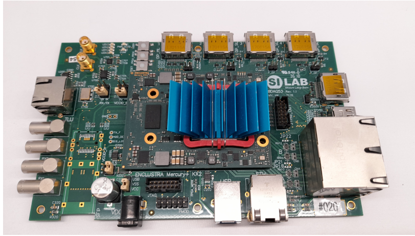
Figure 3.3: BDAQ53 readout board hosting the FPGA daughter board. Picture by Rasmus Partzsch.
