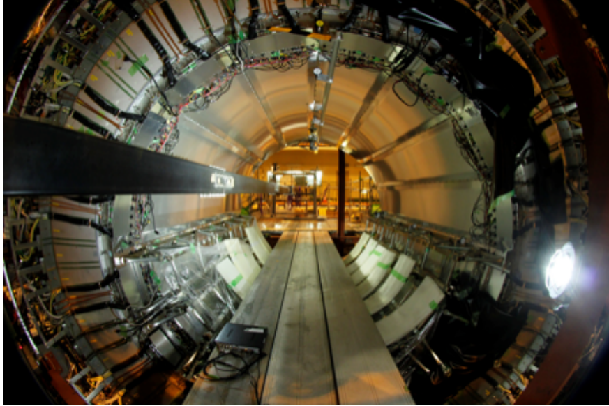
Figure 10: All 16 modules installed in the Magnet in the Belle II experiment
