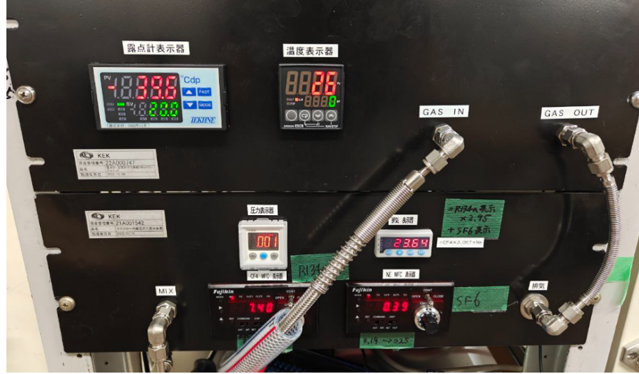
Figure 5.1: Command panel of the gas mixing system. The two symmetrical displays at the bottom are the input thermal mass flow-meters for R134a and SF 6 respectively. The proportion are selected by turning the knobs under the displays. The display in the top-right corner provides the output flow-rate. Other quantities are provided including temperature, pressure and dew point.
