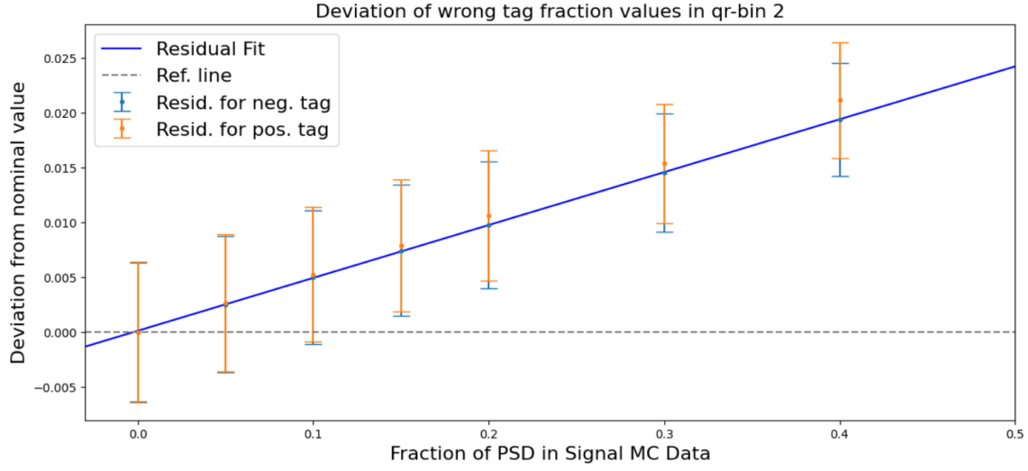
Figure B.15: Relative deviation of fit value with \zeta = 0 from nominal value for parameters w_2^\pm . The dotted line for y = 0 shows the relative nominal value, data points with error bars show data points with respect to the true PSD fraction in Signal MC, while the solid line shows a linear fit to the data points. Wrong tag fraction for negative/positive are shown in blue and orange, respectively.
