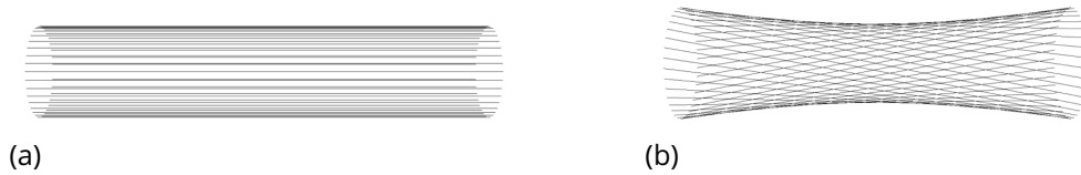
Figure 2.10 – Wire layers of the drift chamber (a) axial : parallel to the beam-pipe, (b) stereo : skewed [83].
