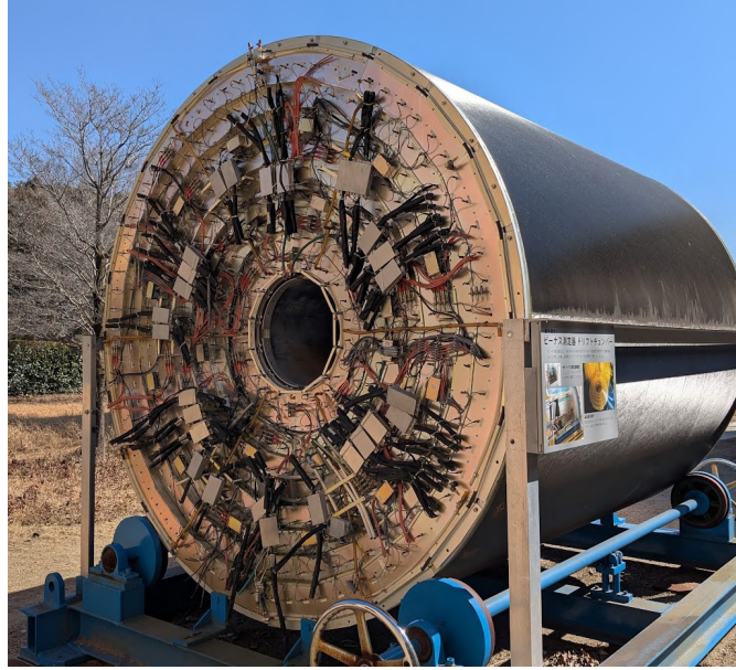
Figure 2.11: Belle Central Drift Chamber (CDC) exhibited at KEK.
