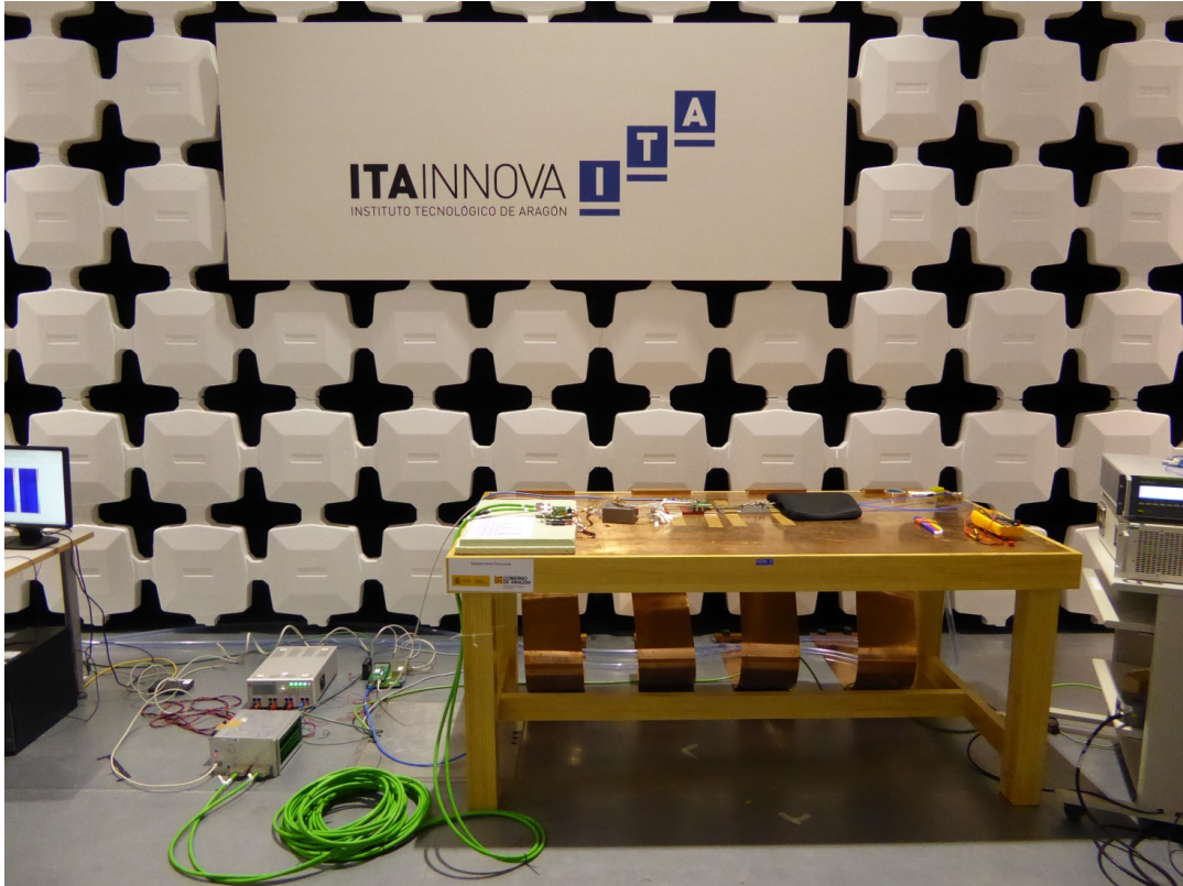
Figure 6.4.: Setup of the EMC measurement campaign of the PXD subdetector inside of the semi-anechoic chamber at ITAINNOVA. The PXD module including the electronics under test were placed on top of a table with a solid copper plane connected to the electrical ground (metallic chamber floor). The auxiliary equipment (power supplies and readout electronics) was placed on the floor next to the table and connected to the PC for control and data analysis.
