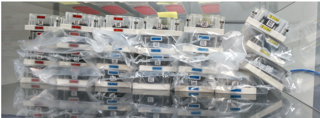
Figure 7.35.: Module storage in nitrogen atmosphere. Every module stays protected in its own transport set. Modules, which are stored for a longer period, are covered in sealed plastic bags for additional protection against dust particles.
