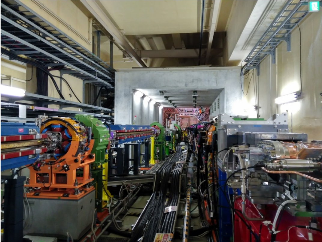
Figure 3.3.: Beam lines north west of Tsukuba Hall facing the detector. The LER (left) containing the positron beam and the HER (right) containing the electron beam cross at the Interaction Point in the center of the Belle II detector which is visible in the back.
