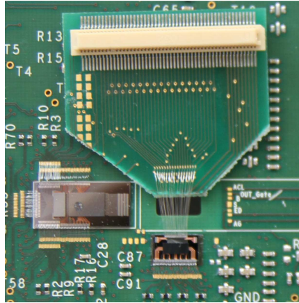
Figure 7-8: Small test board allowing oscilloscope measurements on Switcher outputs.
