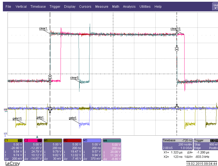
Figure 7-9: Oscilloscope measurement of the Gated Mode with readout. The Clear shifts down to low level on channels currently enabled.
