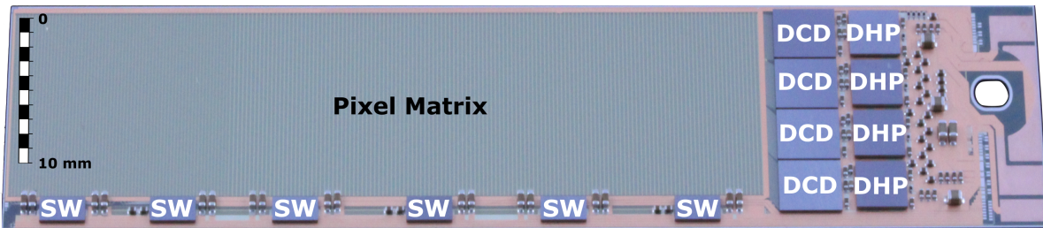
Figure 4.3: Photograph of the PXD9 Pilot module with the full pixel matrix. [26]
