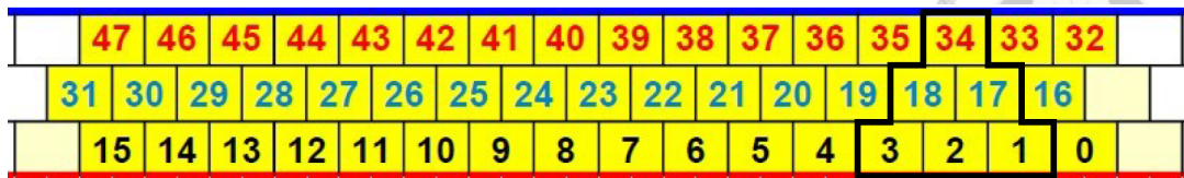
Figure 6.9: Part of CDC outer SL inside wire cell configuration [70].
