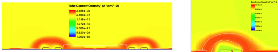
Figure 4.11: Simulated n-side PT effect between two adjacent strips (left) and between a strip and the bias ring (right). Simulation obtained with V_{bias} = 100 V and a voltage difference among adjacent n implants of 25 V.
