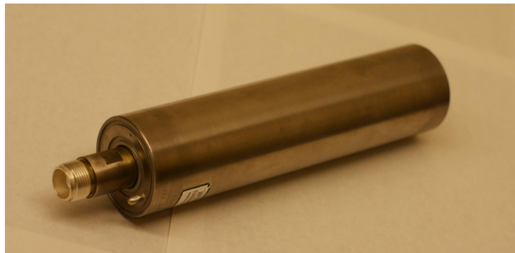
Figure 4.1: Helium-3 tube (see Fig B.1 for a detailed schematic of the detector).
