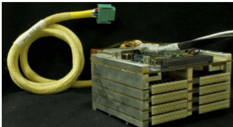
Figure 2.15.: A single electronic readout module, colloquially known as a "boardstack"; the SCROD board in this picture is on top with four carrier boards under, with POGO pin assemblies (two per carrier, eight total); yellow cable is power
