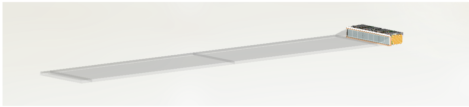
Figure 2.21.: An iTOP module with quartz, MCP-PMTs, and electronics, no QBB
