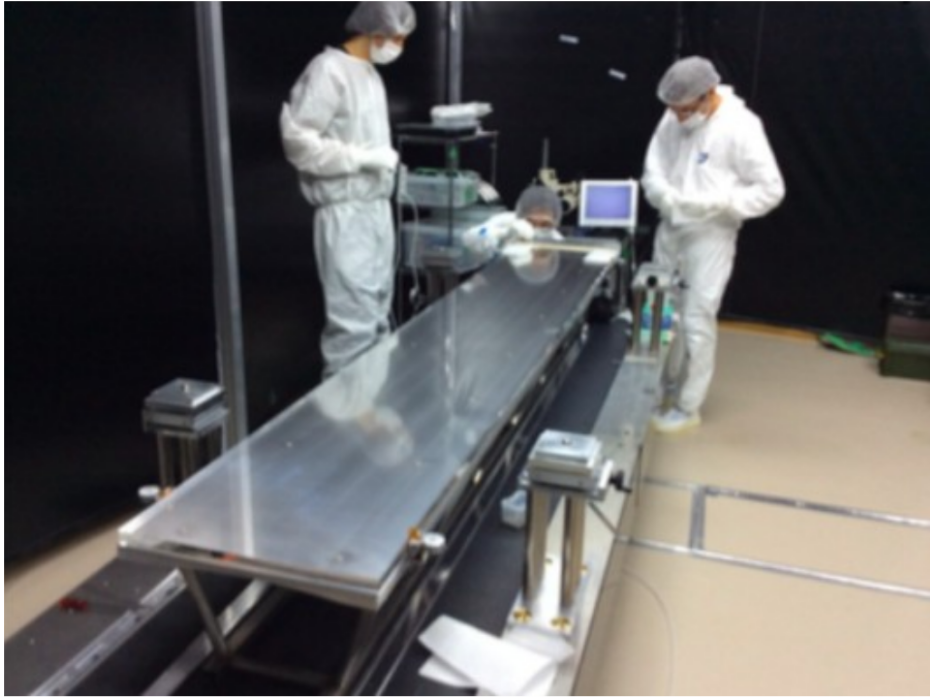
Figure 2.23.: Quartz bar assembly, with QBB, in a clean room at KEK
